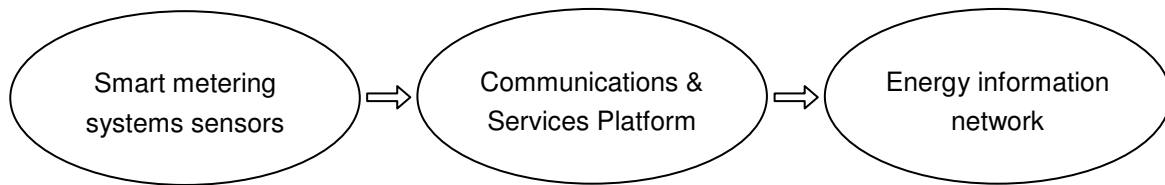
Figure 4: Interaction of basic components for market communication in the smart grid (BDEW)
